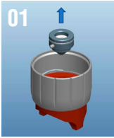
1.- Remove the TIP from the aircap
