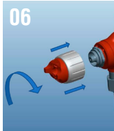
6.- Tighten the aircap tightly until the lip seal is inserted into the nozzle
